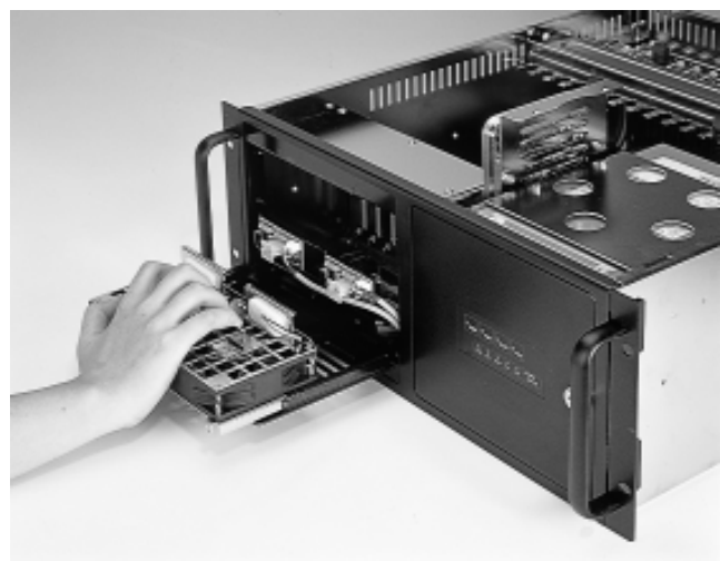
Sliding out the front-access hot-swap fans is easy.
