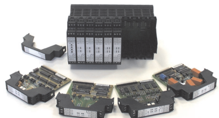
Fig.2 : Basic module RM 213 with 10 sockets for I/O modules
